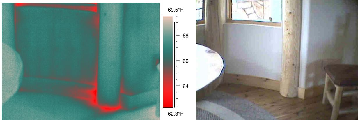
*Figure 11 & 12. – Thermal imaging around log pole that illustrates air infiltration at the base of the pole at interior floor line during the blower door test. Note that half of this poles circumference is exposed on the outside of the wall and the other half creates an exposed log aesthetic on the interior.*
