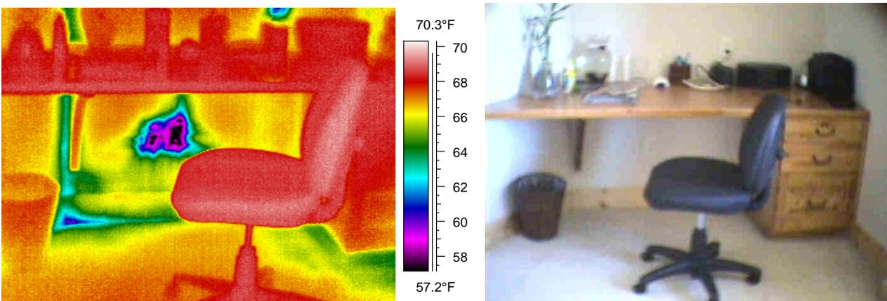
*Figure 17 & 18. - Air infiltration at electrical outlet evidenced by significant cooling of outlet and surrounding materials during the blower door depressurization. Note that this indicates not only that a source for cold air in the logs behind this wall exists, but that the vapor retarder (if present) behind the drywall was not sealed at penetrations such as this outlet.*
