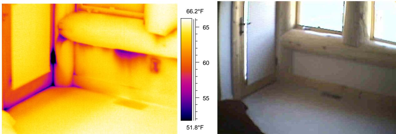
*Figure 13 & 14. – Cooling patterns beneath log under window, at wood-to-wood joinery locations and along doorjamb. Cooling patterns illustrate air infiltration during blower door test. Note there is greater air infiltration under log than at electrical outlet in wall based on temperature differential.*
