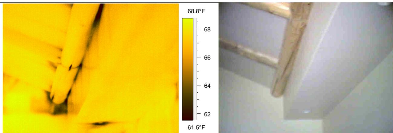
*Figure 23 & 24. – Air infiltration observed as cooling at the end of log beam where it penetrates through the exterior wall, along the length of the beam at the interface with the drywall and at actual splits in the log itself.*
