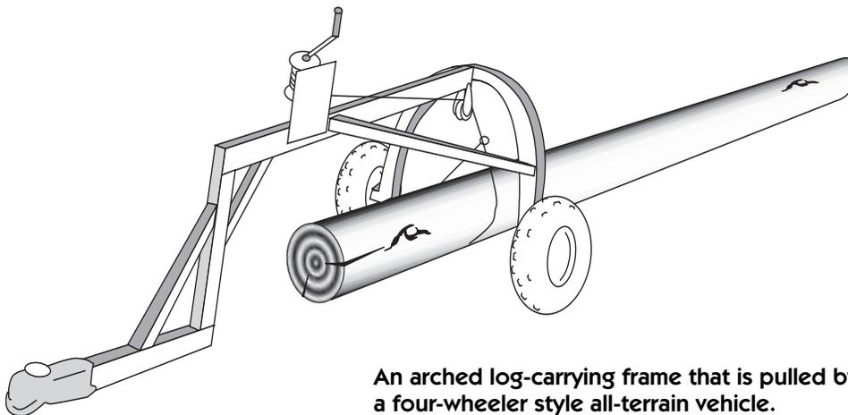
An arched log-carrying frame that is pulled by a four-wheeler style all-terrain vehicle.
