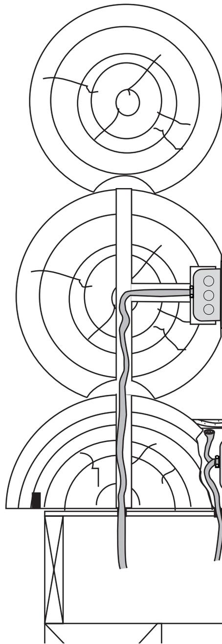
Plan ahead; drill holes for plenty of wires and outlets while building or reassembling walls.
