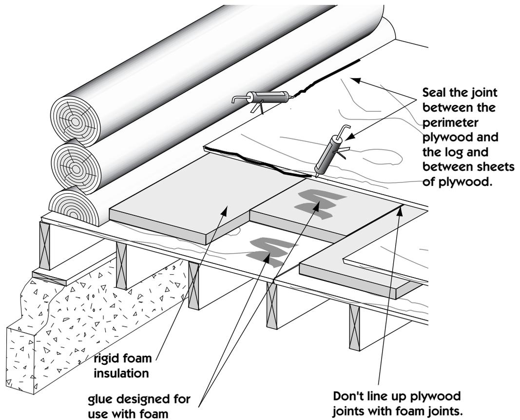
Here is an example of adding rigid foam to the top of the floor without any additional framing. Be sure to stagger the joints of the foam so they don't line up with the joints in the plywood.
