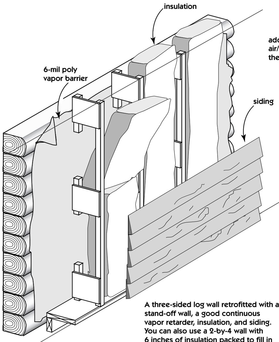
add a Tyvek or other brand air/weather barrier between the insulation and the siding
