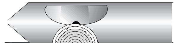
The notch should be smooth and slightly cupped to accommodate insulation and prevent hanging up on the lower log.
