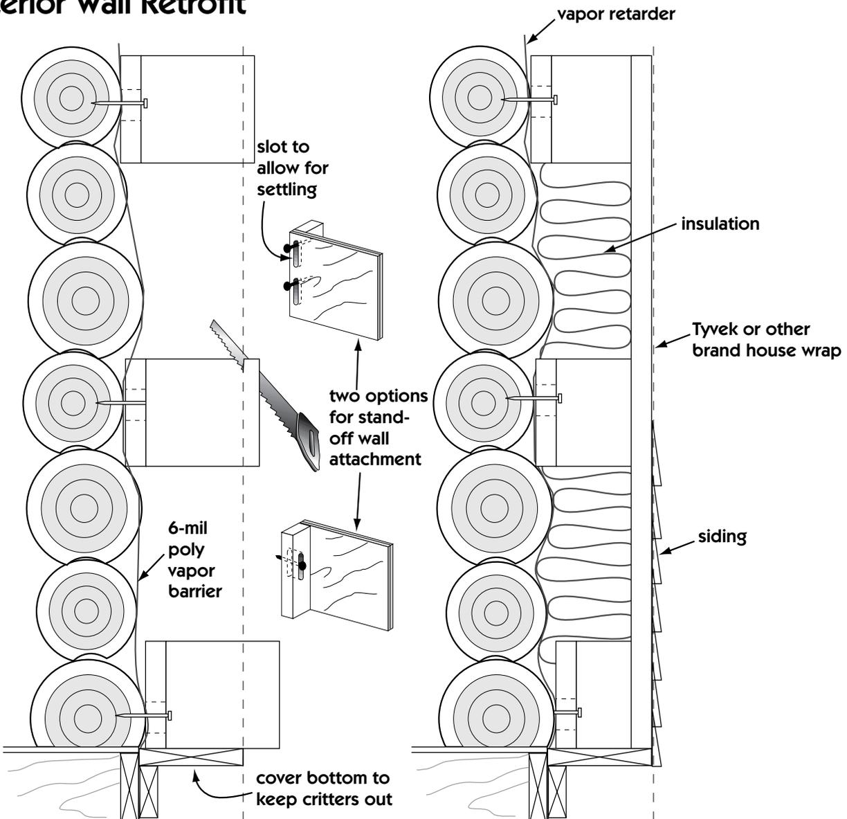
way down and attach the studs and the bottom plate in a manner that will allow for settlement.
