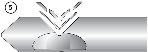
Most of the wood is cut with a chainsaw, but cut the last quarter inch with hand tools.
