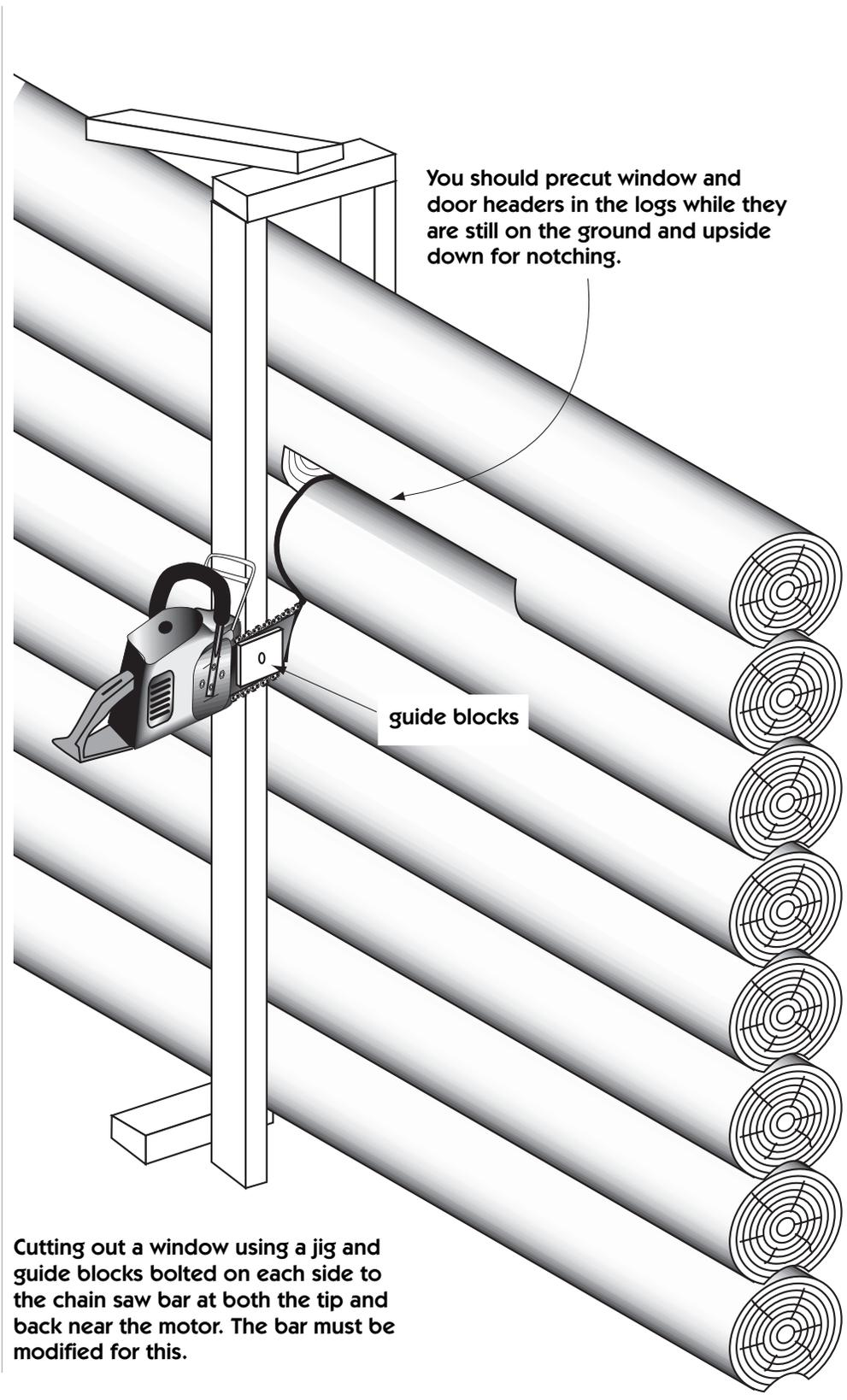
You should precut window and door headers in the logs while they are still on the ground and upside down for notching.
