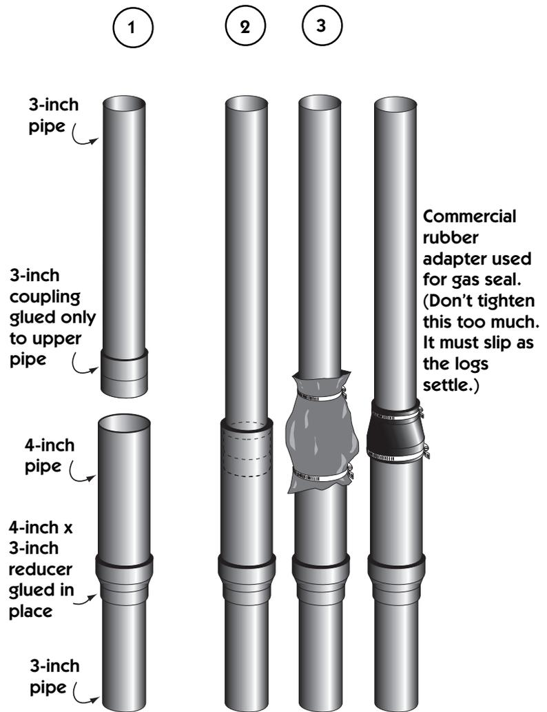
A site-built expansion/settling joint can be made from standard ABS pipe and fittings.
