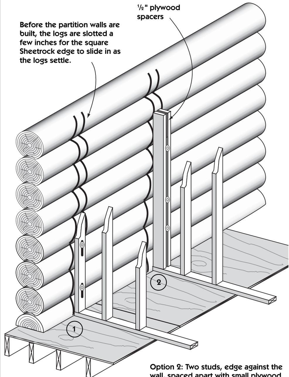
**Option 1:** A stud laid flat against the wall with bolt run through slots long enough to allow for settling. This method uses less wood.
