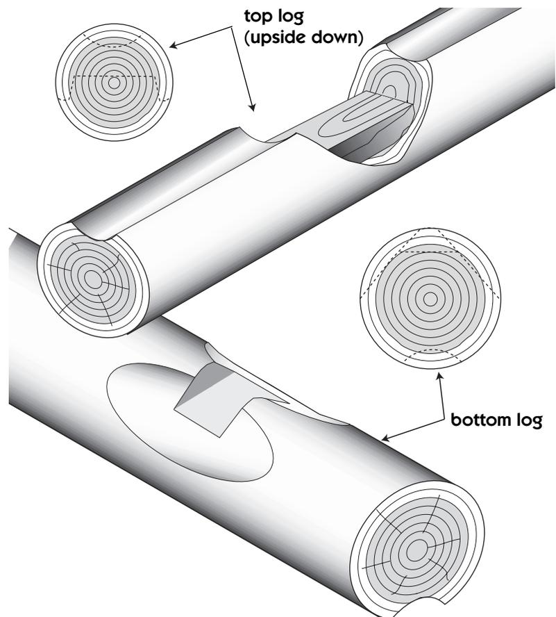
A lock notch is used when a log tip is too small to be notched without weakening it considerably. A lock notch can also be used on the plate log at the top of a wall for added strength to keep the walls from splaying outward.
