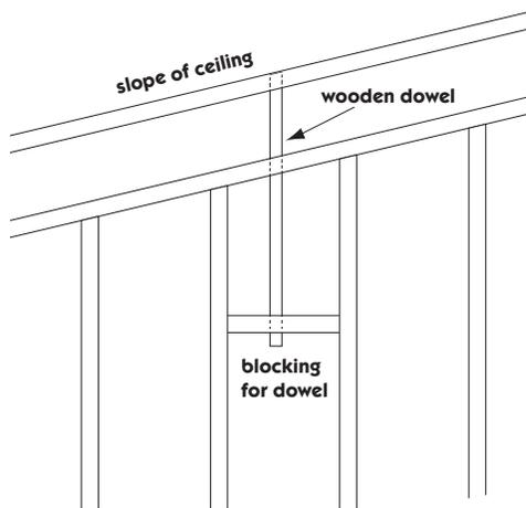
A 2-by-4 stud wall partition slip-joint to keep walls straight and allow the ceiling to settle. A wooden dowel is used to align the partition wall with the top plate, which is attached only at the top. The dowel is run down through snug-fitting holes and braced with additional blocking.
