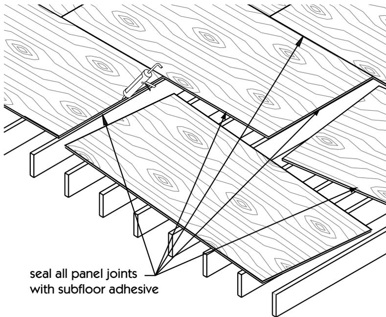
Glue joints between pieces of plywood and glue the plywood to the joists. Ideally, use  $\frac{3}{4}$ " tongue and groove exterior grade plywood. Glue, nail, and screw for a squeak-free floor system.
