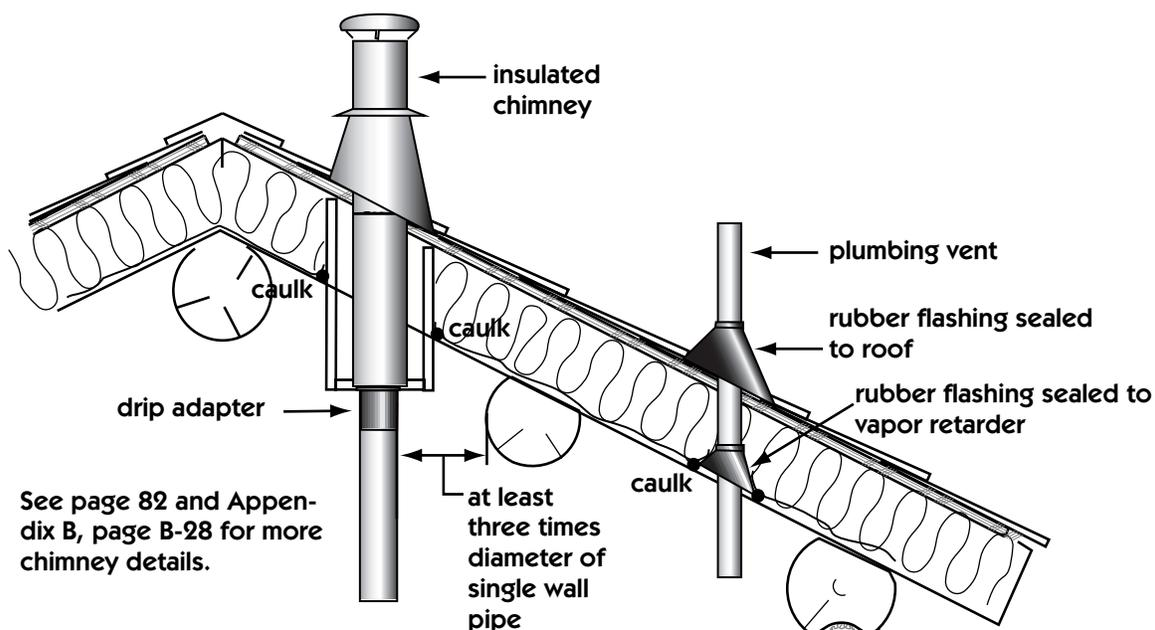
Maintain a minimum 2 inches clearance between an insulated chimney and combustible materials. Single-wall chimneys should be at least three times their diameter away from unprotected combustible materials. Be aware of the possibility of snow sliding on a metal roof and taking the chimney with it or bending it flat against the roof. This could result in a buildup of deadly gases inside the home. Place the chimney near the peak of the roof or protect it with snow stops.
