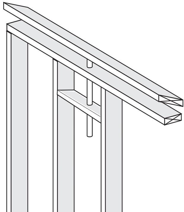
The dowel is only nailed or glued at the top, and slides down through snug-fitting holes in the plate and blocking as the building settles. A 2-by-6 with both sides beveled at ceiling slope and 1 1/2 inches wider than wall frame is nailed or bolted to the ceiling to attach wide crown molding. The crown molding is only nailed at the top and slides down over the Sheetrock.
