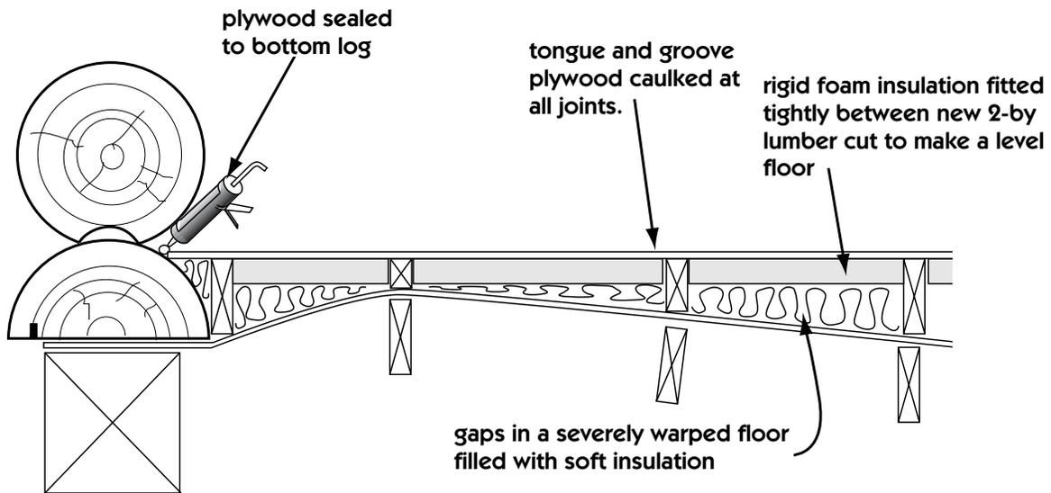
In spite of the insulation cost, it is less labor to install the insulation above the floor than working below the floor, framing additional cavities and making other labor-intensive modifications.
