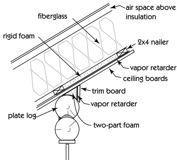
One way to fix the joint between the top wall log and the ceiling is by spraying several inches of a two-part urethane foam into the wedge formed by the wall and ceiling. Then add a vapor barrier (usually polyethylene sealed with an acoustical sealant), and finally cover it with a nice trim board.
