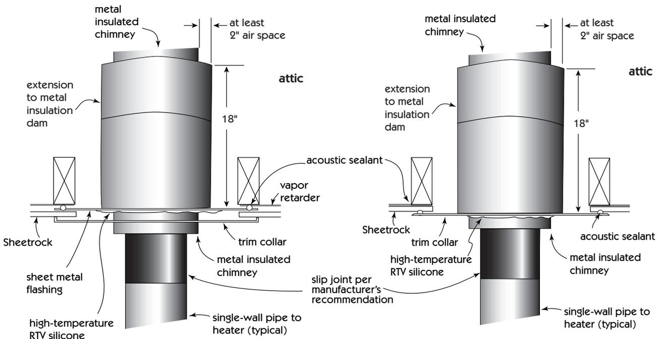
Attic side air seal (typical on new construction)
