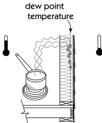
moisture-laden air condenses inside wall, causing damage
