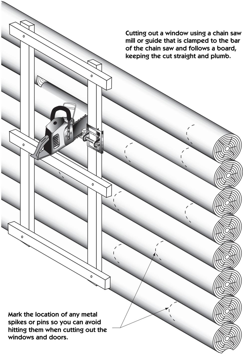
Cutting out a window using a chain saw mill or guide that is clamped to the bar of the chain saw and follows a board, keeping the cut straight and plumb.
