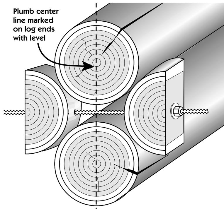
Site-made log holders keep logs aligned at a precut door or window during scribing.
