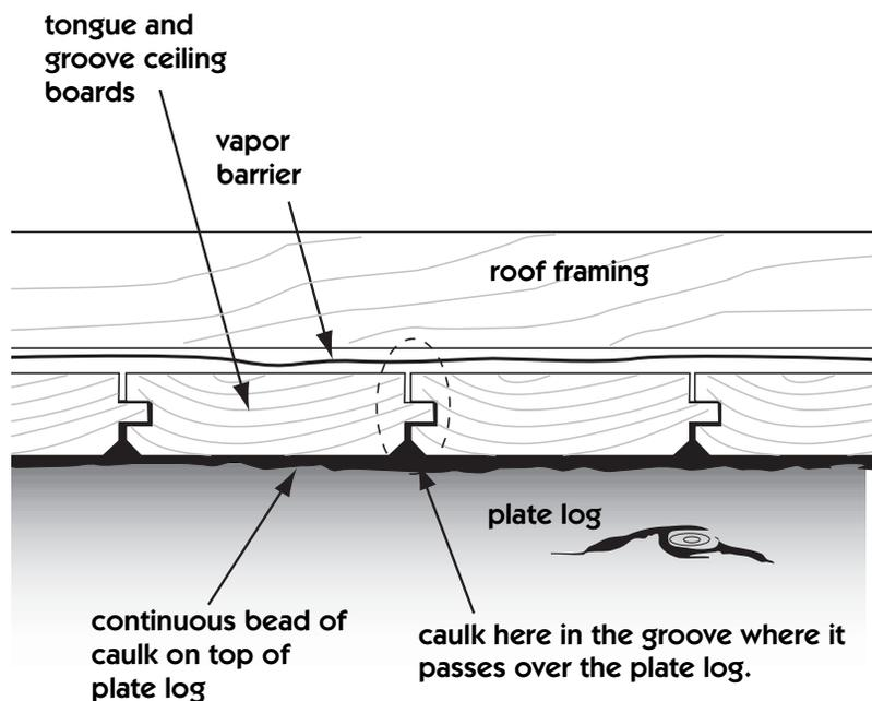
airtight hot roof may be desirable. A number of snow-resistant ventilated roof designs have been experimented with over the years with varying degrees of success. Whatever design you choose, keep in mind that an attic full of snow will not last long. A hot roof must be tightly sealed.
