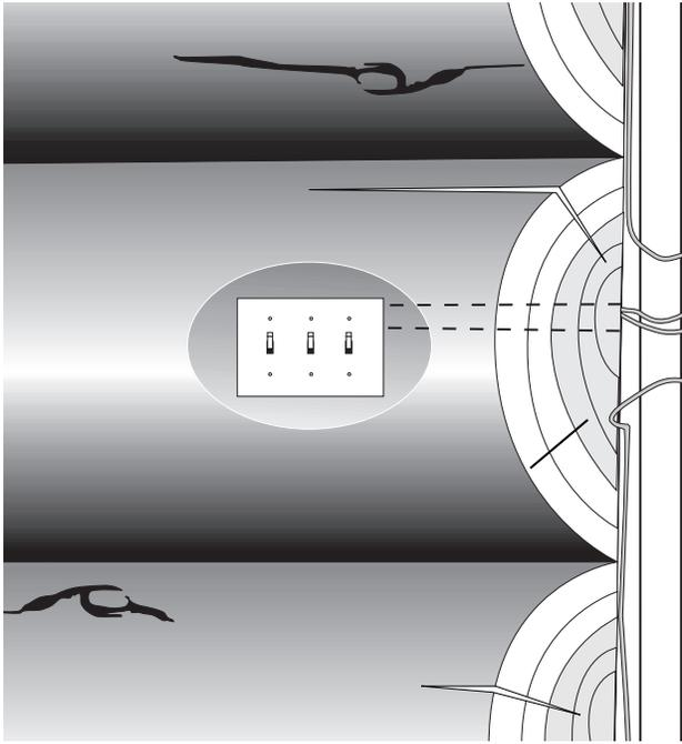
A nicely carved flat spot or scarf is a good way to fit the switch plate cover against the walls. Wiring to switches is often run behind the door spline. Leave slack in the wire for settling.
