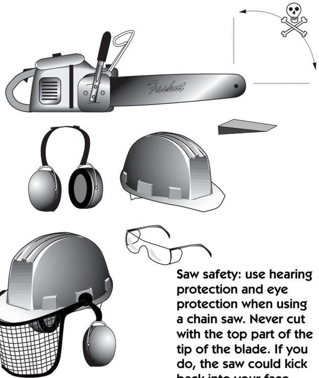
**Saw safety:** use hearing protection and eye protection when using a chain saw. Never cut with the top part of the tip of the blade. If you do, the saw could kick back into your face.
