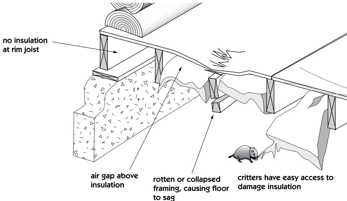
This floor is accessible and has floor joists that are deep enough for the minimum amount of insulation (see Chapter 3).
