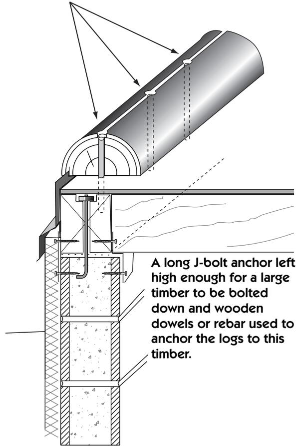
A long J-bolt anchor left high enough for a large timber to be bolted down and wooden dowels or rebar used to anchor the logs to this timber.
