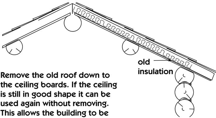
Remove the old roof down to the ceiling boards. If the ceiling is still in good shape it can be used again without removing. This allows the building to be occupied while the roof is being replaced.
