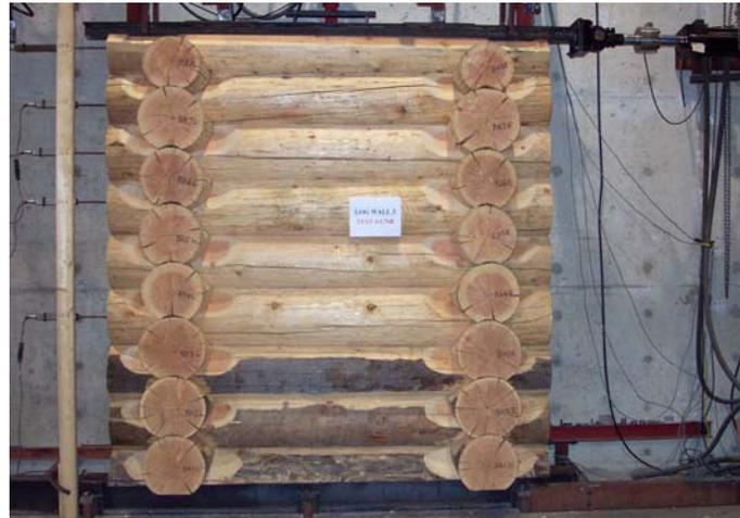
**Figure 17 Handcrafted log wall with corners - setup for the test 4**
