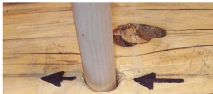
**Figure 13** Wood crushing mechanism around a hole of a pin at the end of test 3
