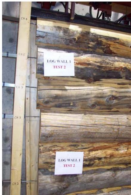
Figure 11 Deformed shape of the wall at the end of the second test
