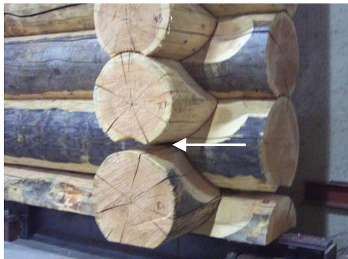
**Figure 32 Gap formation between logs as a result of the uplift forces during test 10**
