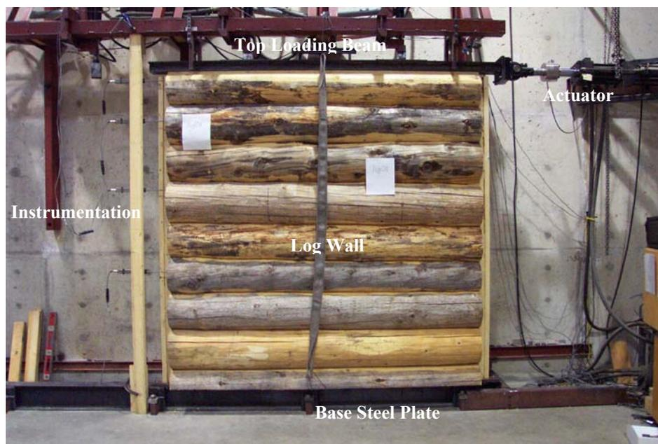
**Figure 1 The lateral load testing apparatus with log wall specimen ready for testing**
