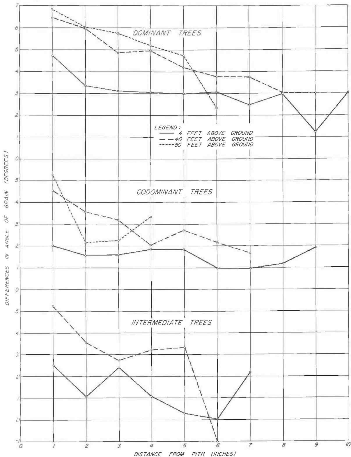
Figure 1. --Average grain angle for successive inches from the pith at three heights in ponderosa pine. Each point represents the average of 6 trees from each of 3 tree classes.
