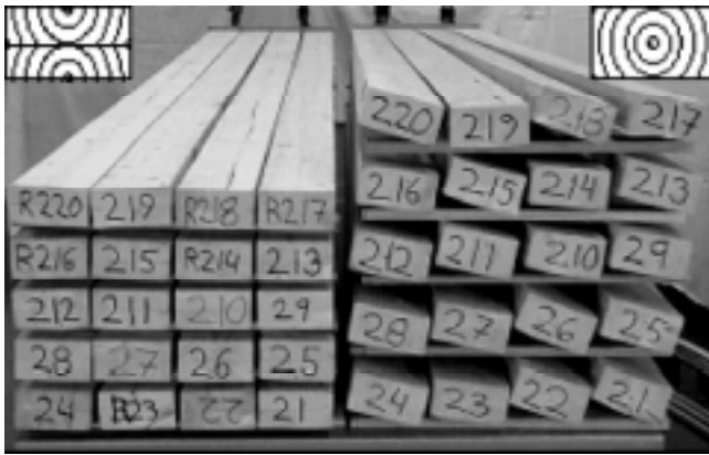
Figure 4. (a) Twist distortions in face to face glued boards (left) and in the control boards (right) at 8% mean moisture content (b) Twist distortions in edge to edge glued boards (left) and in the control boards (right) at 8% mean moisture content
