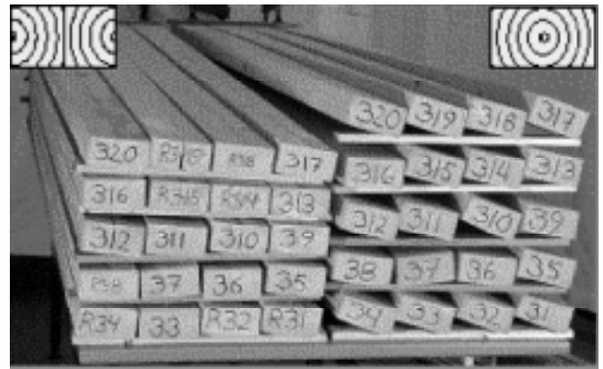
Figure 4. (a) Twist distortions in face to face glued boards (left) and in the control boards (right) at 8% mean moisture content (b) Twist distortions in edge to edge glued boards (left) and in the control boards (right) at 8% mean moisture content
