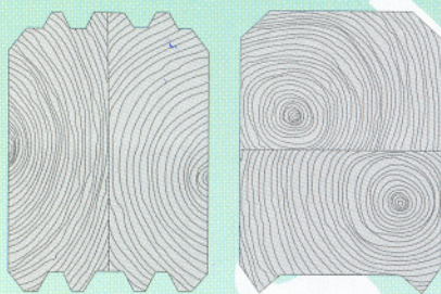
Figure 3. Profile of a glued log (vertical and horizontal)
